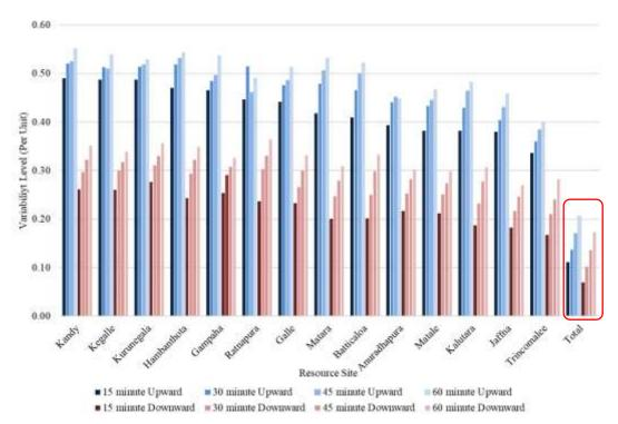
A5.6 Solar PV variability levels (15min, 30min, 45min, 60 min) of power outputs of different sites and total power output based actual data covering the country
