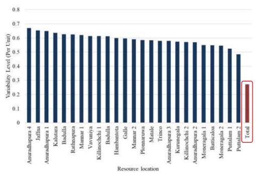
A5.7 Solar PV variability levels (60 min) of power outputs of different sites and total power output based on satellite data covering the country
