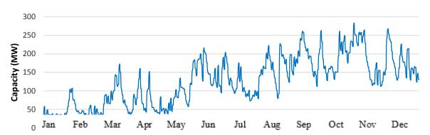
A5.4 Modelled production profile of Minihydro resource based on 2017 data
