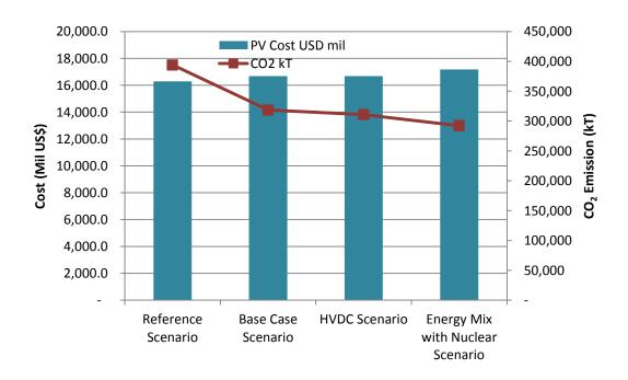
Figure 10.10 - Comparison of System Cost with CO<sub>2</sub> Emissions
