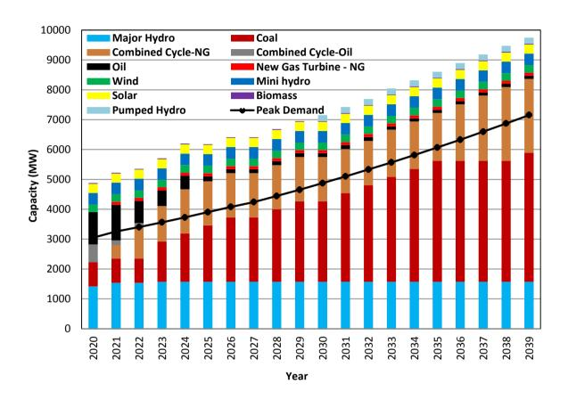
Table 7.1 - Cumulative Capacity by Plant Type in Reference Case
