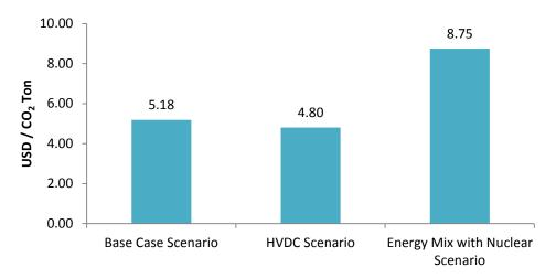
Figure 10.11 - Comparison of Incremental Cost for CO<sub>2</sub> reduction
