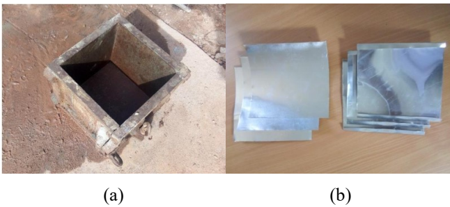
Fig. 1. Test specimen mold fabrication: (a) mold and (b) measurement terminals.
