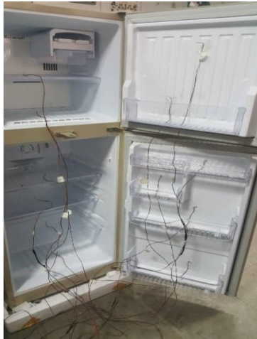
Fig. 1. Thermocouple arrangement of empty refrigerator.
