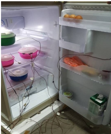
Fig. 2. Thermocouple arrangement of refrigerator loaded with food.
