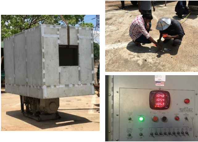
Fig. 2. Fabricated enclosure and sound pressure measurements.
