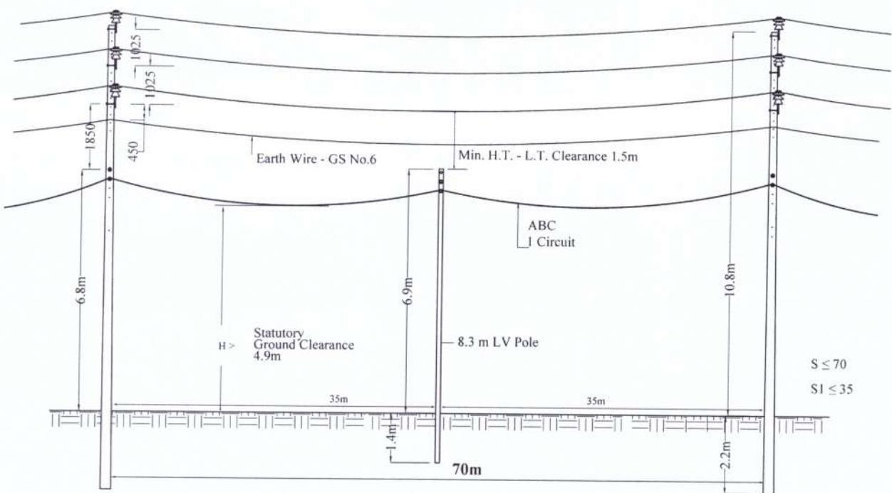
13m Pole Combined Run 33 kV double circuit and LV with Intermediate LV Pole ( Accessible to Traffic )
