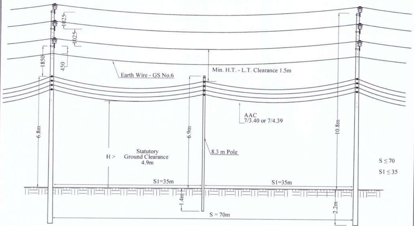
13m Pole Combined Run 33 kV Double Circuit and LV Line with Intermediate LV Pole Across the Road
