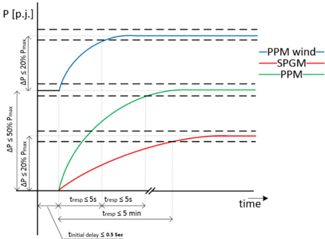
Figure 3.17- 2: Active power upward ramping rates
