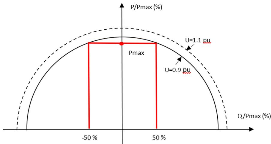
Figure 3.17- 4: Steady state active and reactive power limits
