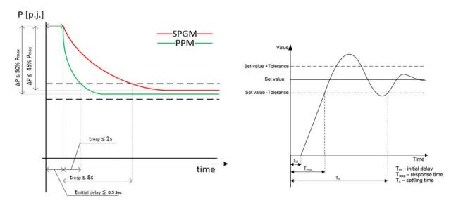
*Figure 3.17- 3: Active power downward ramping rates [SPGM: synchronous power generation modules]*
