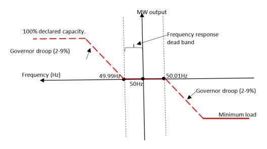
Figure 3.17- 5: Typical FSM settings
