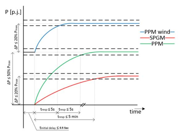
Figure 3.17- 2: Active power upward ramping rates
