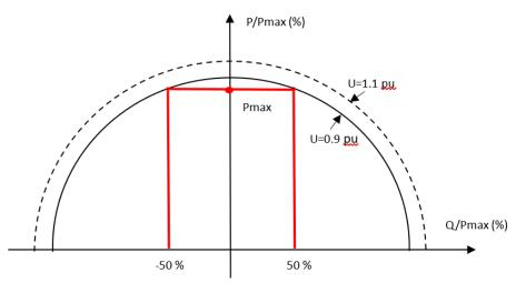
Figure 3.17- 4: Steady state active and reactive power limits
