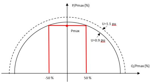
Figure 3.17- 9: P-Q capability that can be specified for power park module
