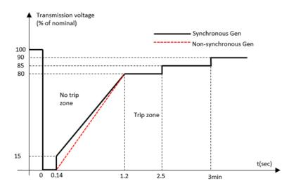
Figure 3.17- 10: Fault Ride Through requirement - Voltage duration curve
