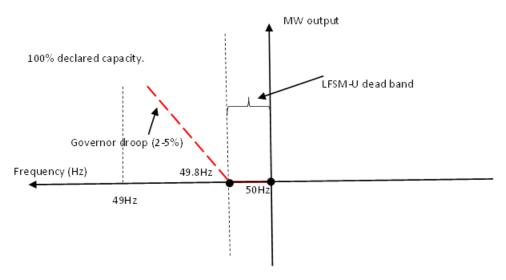
Figure 3.17- 7: Typical LFSM-U settings
