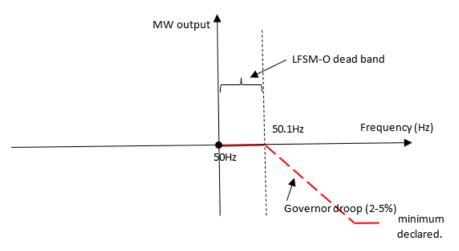
Figure 3.17- 6: Typical LFSM-O settings
